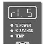
After 20 seconds of keypad inactivity, the control will return to the normal display.
