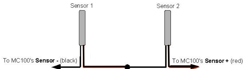
Diagram for connecting two temperature sensors to the MC100.
